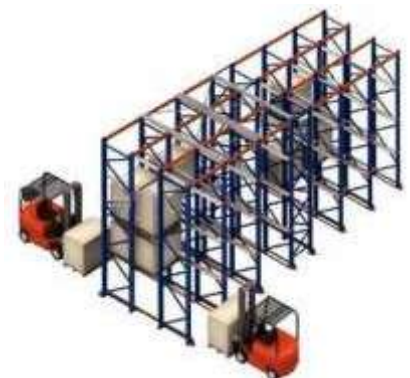
Drive in Racking System
